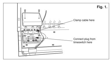
Replace the electrical box cover, splash cover and fascia bottom panel, and secure the fascia using the two screws and refit the front panel.
